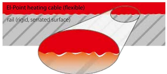
Due to its flexibility, the heating cable can equalise most of the rails irregularities. Thus the **heat transfer into the rail is enhanced** and results in a higher rail temperature at relatively low energy consumption.
