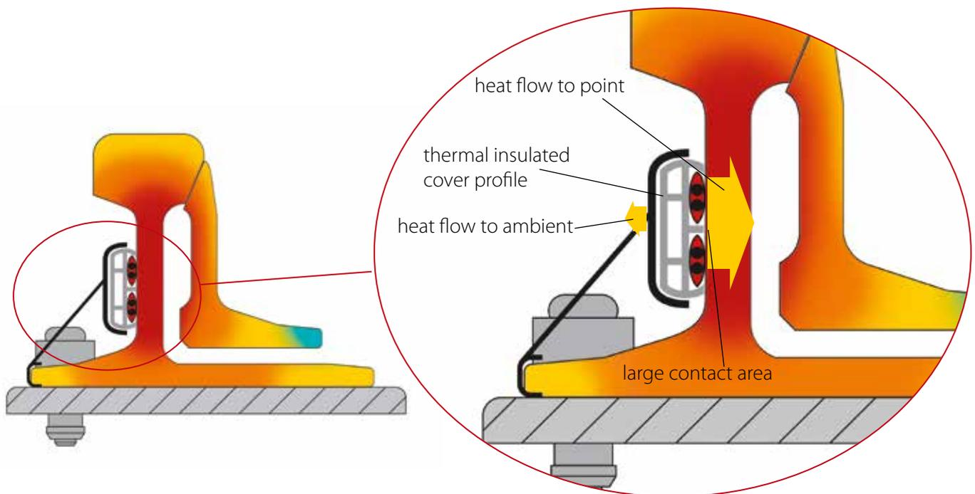
The thermally insulating cover profile reduces heat losses to ambient and directs the heat flow toward the rail. The big, dark rail surface turns into a radiator - the heat radiation frees the gap between stock rail and switch-
