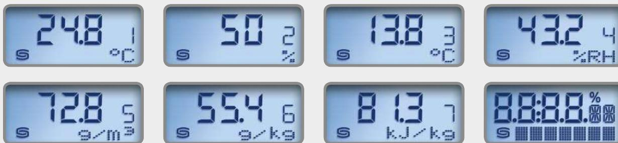
By default, the display alternates between the **actual temperature** and the **actual humidity** (relative humidity). For improved legibility, backlighting is provided.
