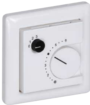
FSTF xx PD4 Version with sensor, potentiometer (1 kOhm, max. 0.1 W) and turn switch (max. 24 V AC / DC, max. 130 mA)
