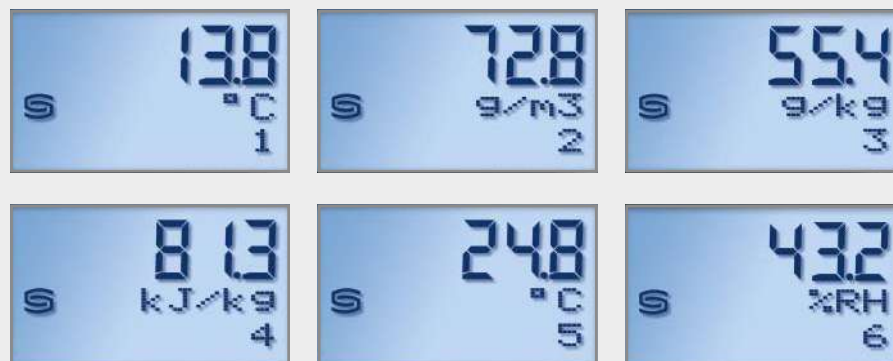
Display screen (static) alternative output variables
