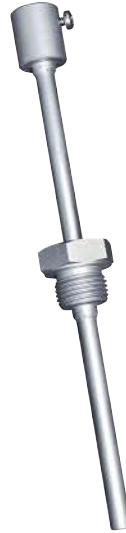
TH08-VA/xx/90 Immersion sleeve with neck tube, stainless steel, V4A, flat-sealing, cylindrical, according to DIN 228
