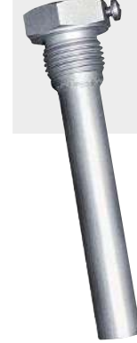
THR -VA-17 / xx Immersion sleeve, stainless steel V4A (1.4571) flat sealing, cylindrical, according to DIN 228
